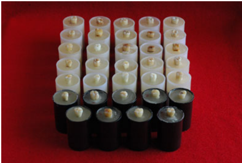
Fig 1. Sample teeth used for shear bond testing.
