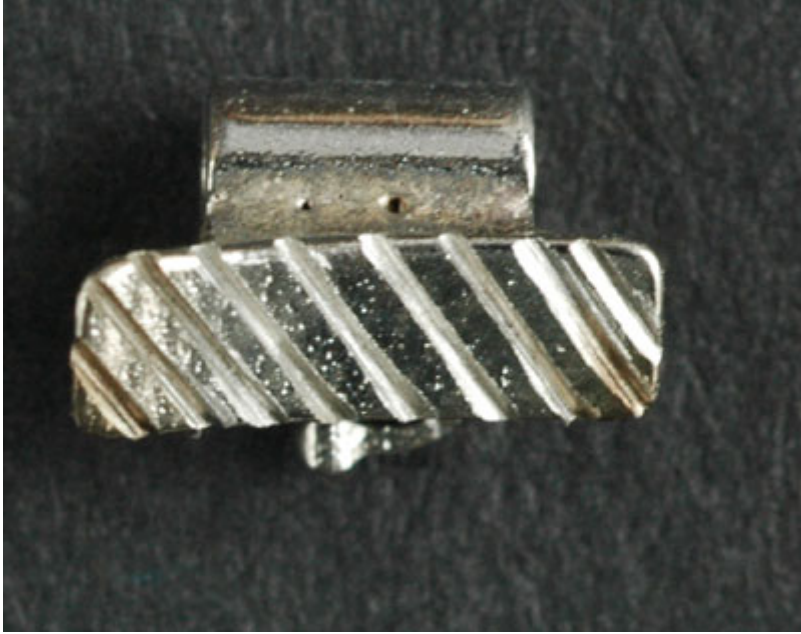
Fig 2-B Making seven to nine oblique grooves on the base.
