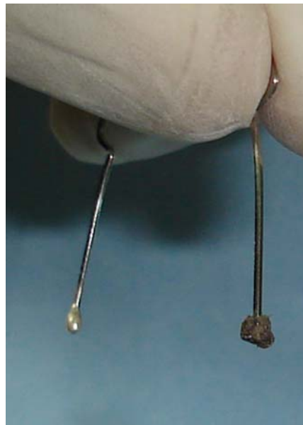
Figure 1. Silver solder paste with flux is applied to the distal end of the archwire.
