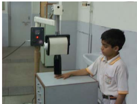
FIGURE 1. Method of Recording MP3 Radiograph using dental Intraoral Periapical X-ray Film.
